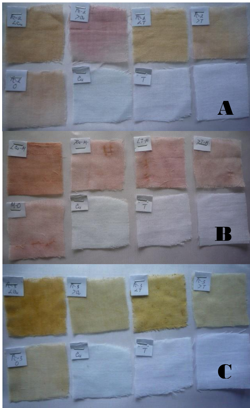
Figure 3. Dyed clothes with natural dye from Penicillium sp. strain R-3 (A), Monascus purpureus (B), and Penicillium sp. strain RC-1 (C). < = pre-mordanting; > = post-mordanting; Cu = \text{CuSO}_4 \cdot 5\text{H}_2\text{O} ; T = alum; O = without mordanting
